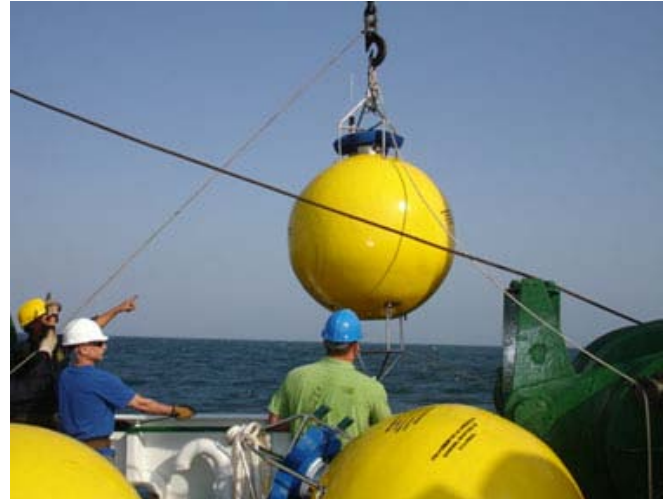
Deployment of sub-surface 75 khz ADCP as a component part of the three taut wire moorings
